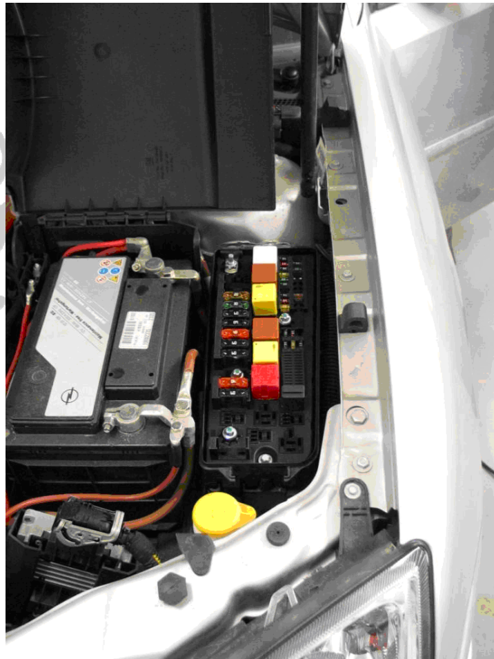
Figure 3.1b Under-hood Electrical Center (UEC)
