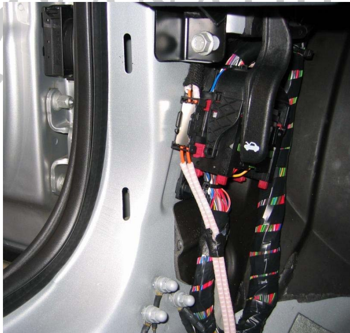
Figure 9.1d BCM mounted on IPBEC.
